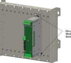
Mount RS485 Networking Module with two M6 x 10 Screws provided with module.
